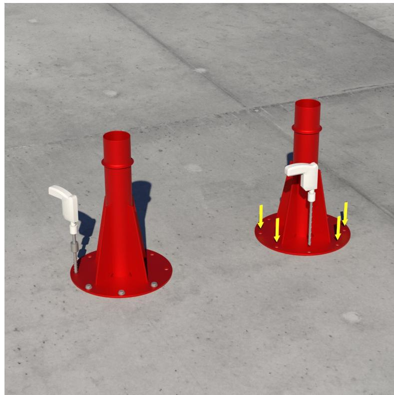
The ceiling socket is installed using eight HUS 10x100 concrete screws.
