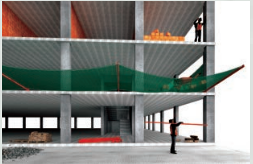
LiteMESH module in top mount configuration.
