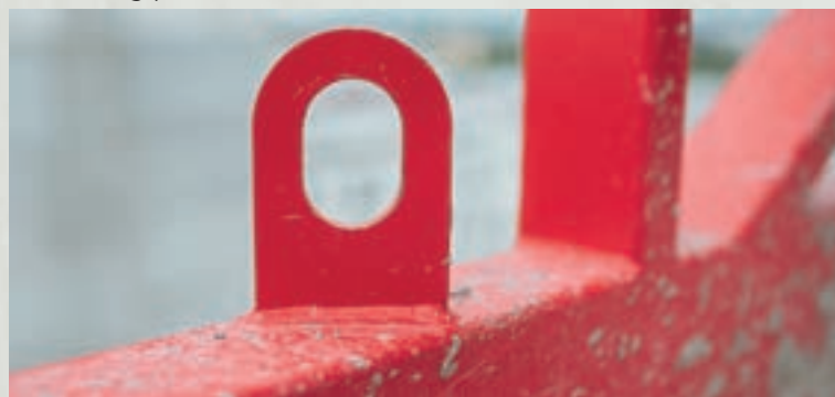
Fixing of the crane's sling
