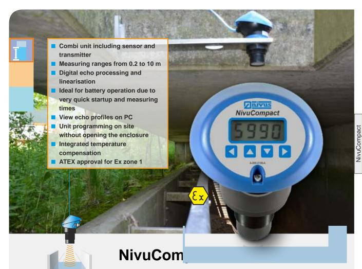
Ultrasonic compact echo sounder as 2- and 3-wire system for non-contact measurement of level, distance, empty space or volume. Parameters can be set directly on site without the need to open the enclosure.
